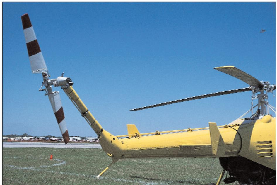
**VAT moved the horizontal stabilizers forward to minimize rotor downwash and to gain improved control balance as a result.**
