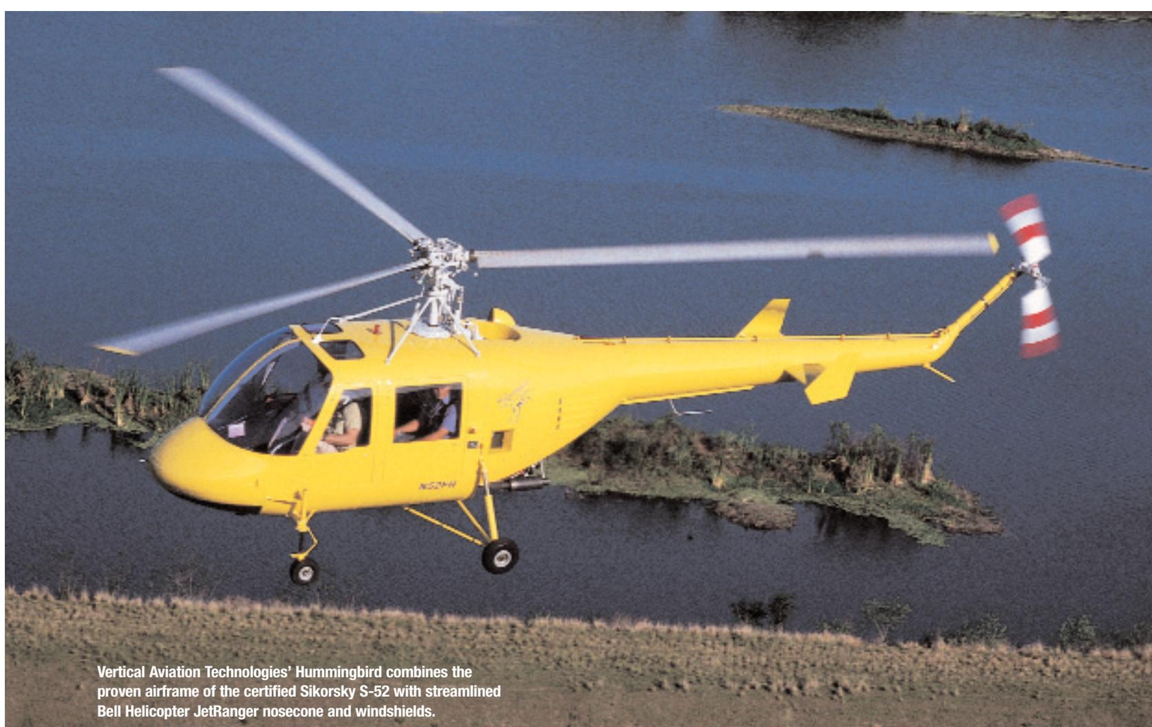
Vertical Aviation Technologies' Hummingbird combines the proven airframe of the certified Sikorsky S-52 with streamlined Bell Helicopter JetRanger nosecone and windshields.
