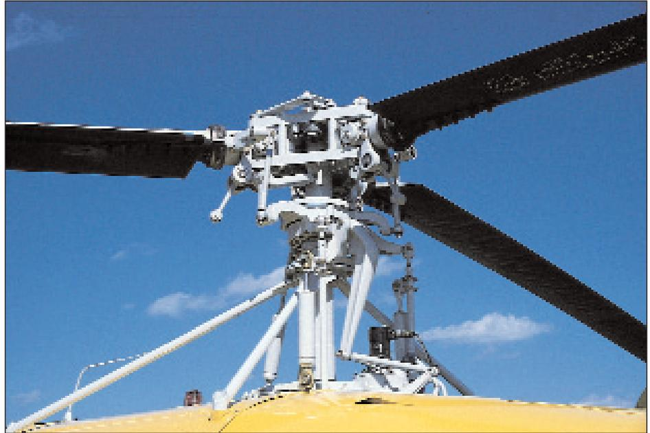
**The rotor blades were modernized by VAT, and a significant reduction in rotor vibration (compared to the S-52) resulted.**
