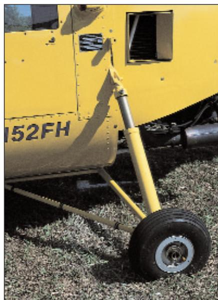
The Hummingbird landing gear is equipped with wheels rather than skids, a feature that offers improved flexibility and performance during takeoff, landing and taxi operations.
