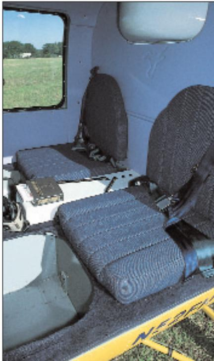
**Two rear seats make the Hummingbird the first four-place kit helicopter commercially available. The 900-pound useful load allows for four 170-pound occupants and about 36 gallons of fuel.**
