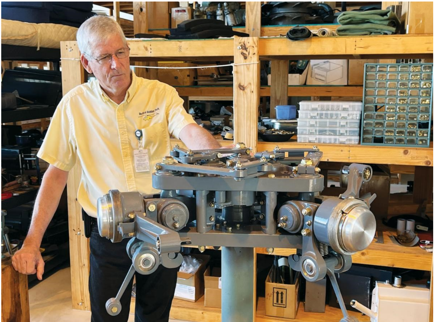
Brad Clark, owner of Vertical Aviation Technologies, shows the Hummingbird's rotor hub in the form delivered to kit builders. It is fully primed and assembled, ready to mount. Big, too.
